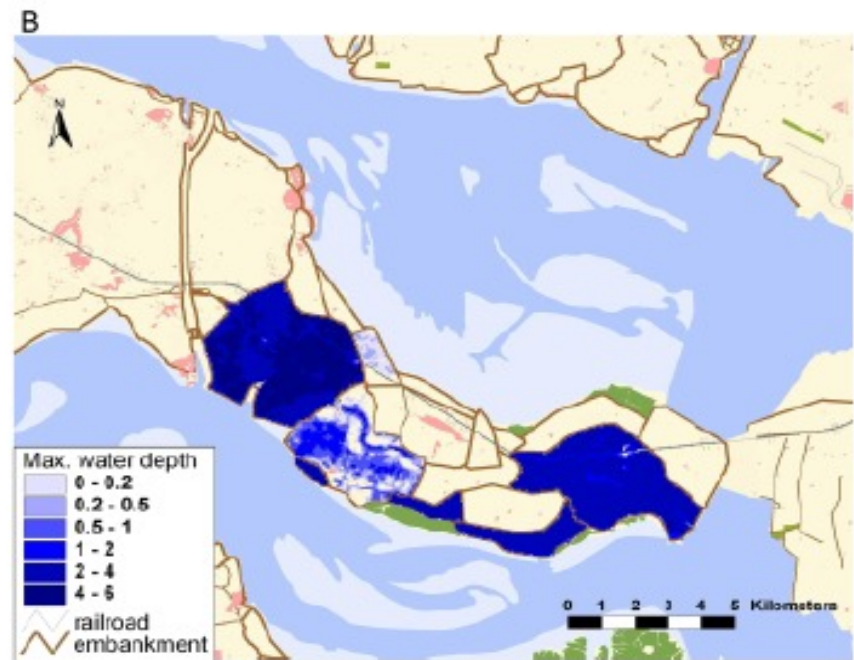
Figure 2 Areas flooded in a dike-ring area in the southwest Netherlands during the 1953 disaster (a) and flood pattern and depth resulting from breaches in the same locations as simulated with SOBEK 1D-2D (b), both showing the influence of former flood defences on flooded surface area
